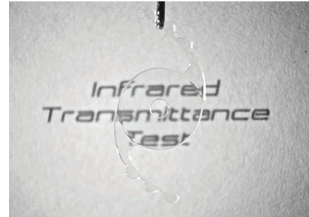
Figure 5. The black acrylic material is transparent to infrared light, allowing examination of structures located behind the implant using infrared-based equipment.
